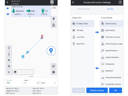
With graphic display, now it is easy to you to observe the relation between occupied point and target points. It will help you to make less mistakes when measuring many points.
