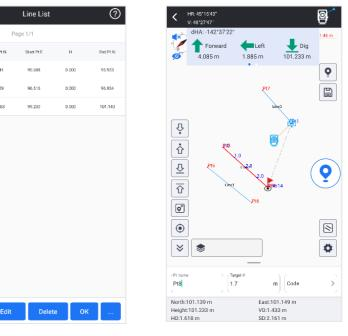
User is allowed to manually choose points from library, line will be formed by program automatically. Then user input interval distance, setout points will be calculated out and displayed on screen.
