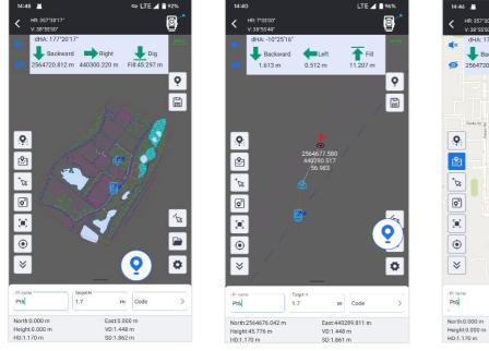
CAD Stakeout allows you to import CAD basemap and stakeout it, without input point coordinates one by one.
